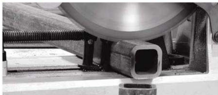
Carbide-Tipped Blades make Virtually Spark-Free Cuts
